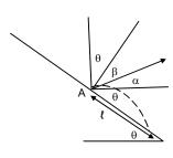
Using equation of trajectory, y = x tan  $\alpha - \frac{gx^2 \sec^2 \alpha}{2u^2}$
